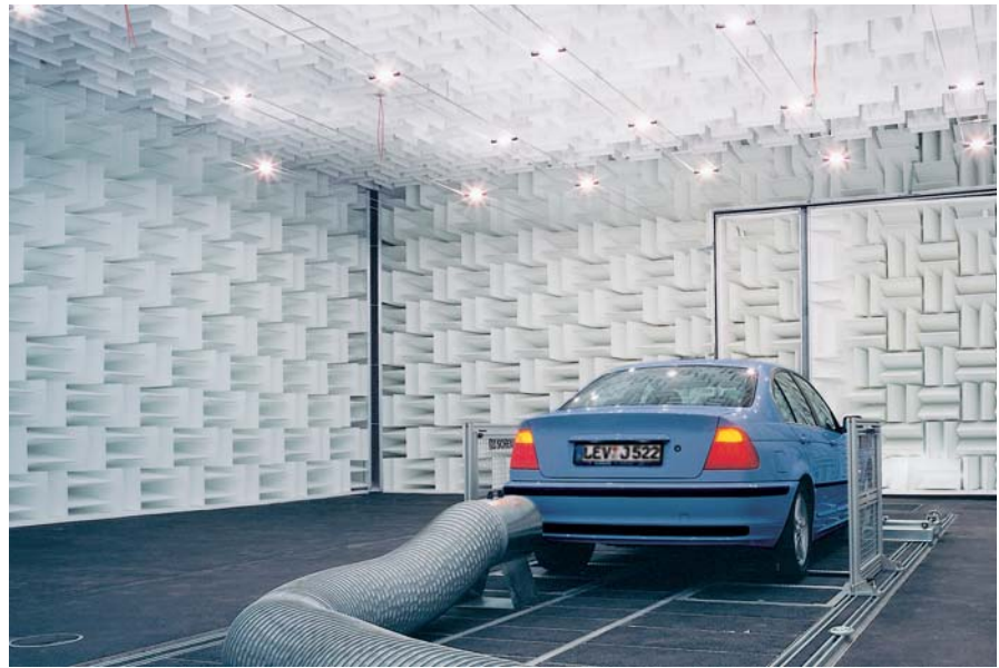
SONEX Wedges can be used to create full anechoic or hemi-anechoic chambers.
