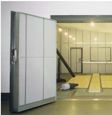
Hemi-anechoic chamber at Continental Brakes in Hannover, Germany contains the SONEXtrilayer System with SONEXflat™ Panels.
